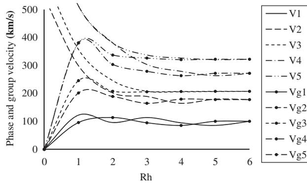
Fig. 5. Phase and group velocities of flexural modes in non-conducting (isentropic) elastic plate versus wavenumber ( $Rh$ ).
