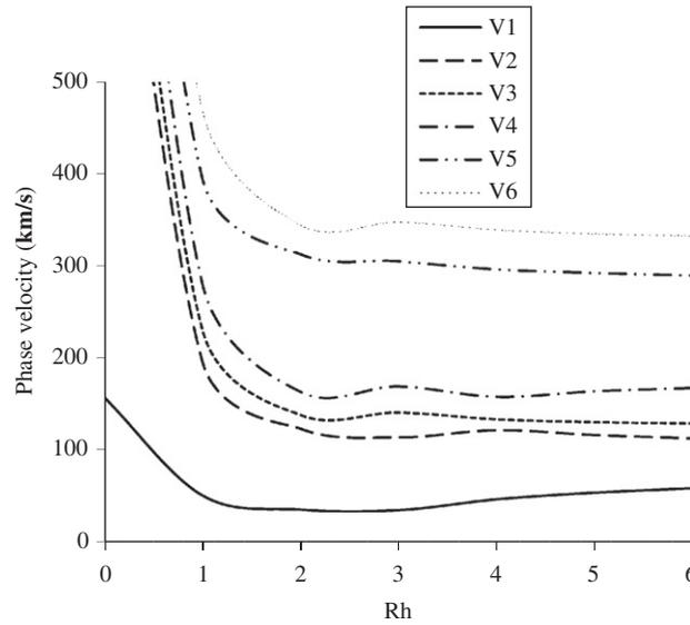
Fig. 3. Phase velocity of extensional modes versus wavenumber ( $Rh$ ) for CT theory.
