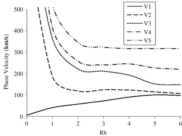
Fig. 7. Phase velocity of flexural modes versus wavenumber ( $Rh$ ) for CT theory.
