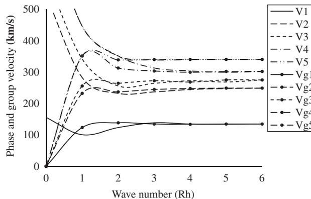
**Fig. 1.** Phase and group velocities of extensional modes in isothermal elastic plate versus wavenumber ( $Rh$ ).
