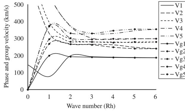
Fig. 2. Phase and group velocities of extensional modes in non-conducting (isentropic) elastic plate versus wavenumber ( $Rh$ ).
