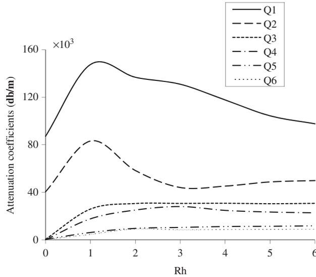
Fig. 9. Attenuation coefficients of extensional motion versus wavenumber ( $Rh$ ) for CT theory.
