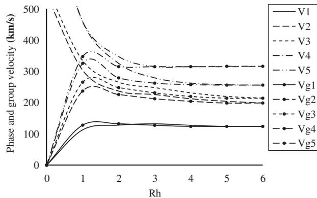
Fig. 6. Phase and group velocities of flexural modes in isothermal elastic plate versus wavenumber ( $Rh$ ).
