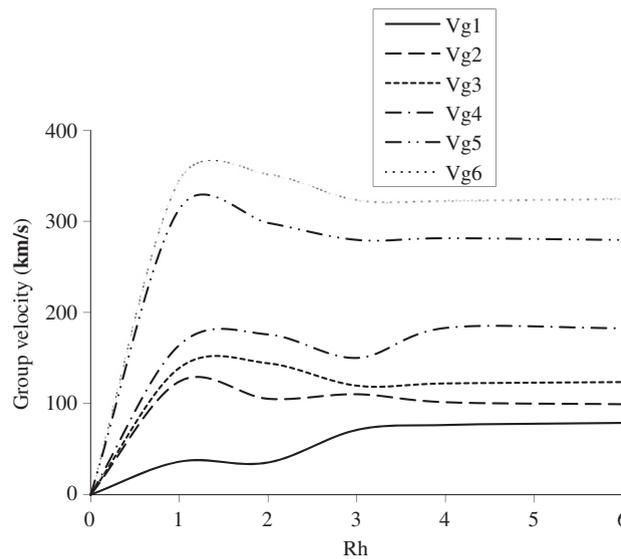
Fig. 4. Group velocity of extensional modes versus wavenumber ( $Rh$ ) for CT theory.
