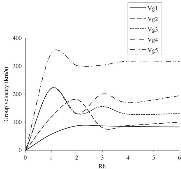
Fig. 8. Group velocity of flexural modes versus wavenumber ( $Rh$ ) for CT theory.
