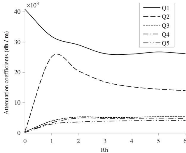
Fig. 10. Attenuation coefficients of flexural motion versus wavenumber ( $Rh$ ) for CT theory.
